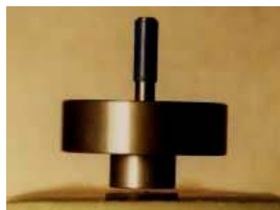
Picture 2. : Demonstration of the great levitation force
